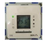
If you push both  $\blacktriangle$  &  $\blacktriangledown$  buttons briefly, the display will change to show the actual floor temperature. Release both buttons & the air temp will again be displayed. Press & hold both the  $\blacktriangle$  &  $\blacktriangledown$  buttons for more than 2 seconds and the display will revert to displaying the actual floor temperature.
